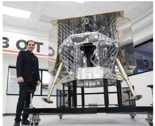
Ander Solorzano, Astrobotic Systems Engineer, stands beside the Peregrine Structural Test Model.
